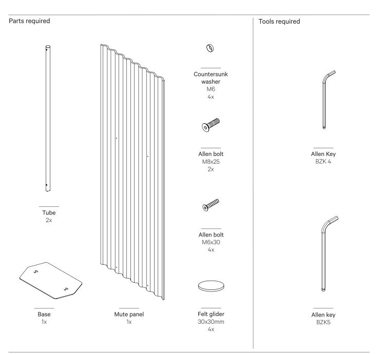
1 Fit both tubes into the base and bolt it tight with the M8x25 allen bolt. Place the felt gliders on the bottom of the base (4x).
