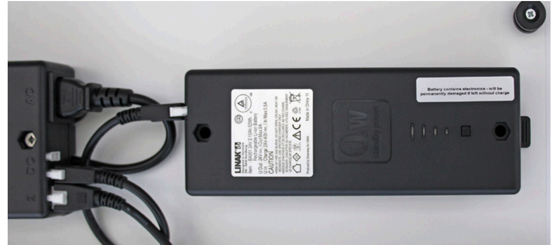
The optional battery is just clipped into the holder underneath the table top.
