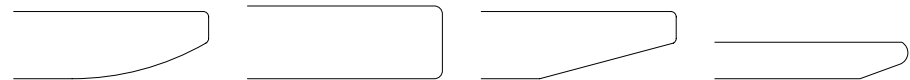
Solid wood lipping, rounded on the bottom, straight plastic lipping, chamfered wood lipping or chamfered HPL solid-core lipping
